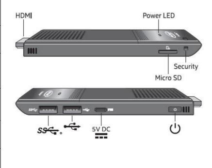
First, you will want to unwrap all materials and remove the safety cap from the HDMI connector. After all materials are out, connect the HDMI of the QStick™ to the Monitors/Kiosks QHDMI adapter.
