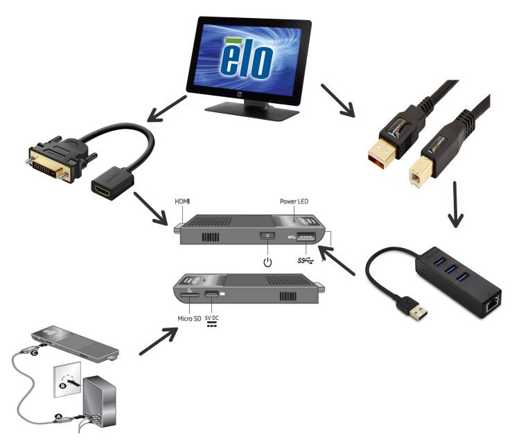
Thats It!, The intel Compute stick should power on with a BLUE led indicator, and the touchscren should turn on as well and beign to boot. Once online Simply login with your given Kiosk Username and password and you should be good to go!
