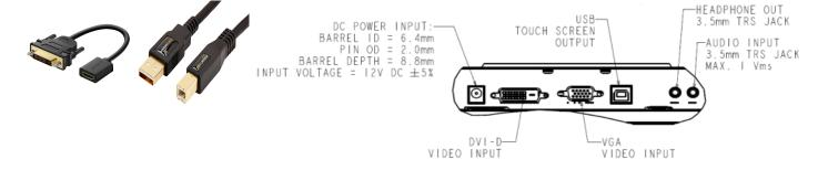
2. Connect the Intel Compute Stick (Qstick) To the CableMatters or Anker USb Hub, via its USB Connector on the left side, and connect the Intel Compute sticks HDMI port (hidden under a cap) to the DVI to Female HDMI Connection you attached earlier to the monitor. Then Route the USB cable coming from the monitor (USB A - B) to one of the USB connectors on the Cable Matters/Anker USB Hub.
